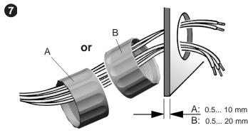
For 52 mm instruments, the fastening nut can be mounted at position A or B. This allows you to realize various clamping heights.
