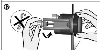
Place the bracket on the stud bolt and hand-tighten the knurled nut.
