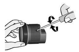
The gauge must be calibrated to the connected immersion tube sensor. Adjust the setting with an insulated screwdriver when the tank is **empty**. Rotate the potentiometer until the gauge reads empty (0 or E).
