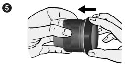
Place the new front ring on the instrument and press it on until it is flush with the instrument glass.
