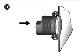
Place the flush mount seal A2C53215640 on the instrument glass.
