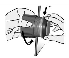
Align the instrument and hand-tighten the fastening nut. Ensure that the nut is not tightened with a torque greater than 400 Ncm.
