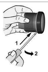
If the instrument is mounted flush (i.e., from the back so that the instrument glass and the panel form one plane), the front ring must be removed. Press the instrument glass with both thumbs, while at the same time pressing the front ring forward from the instrument with both index fingers. Note the use of a tool in the adjacent figure.
