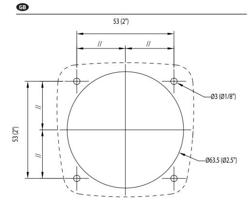
The panel has a pre-installed seal and is secured with the 4x screws included in the packaging (See Fig 3.2)
