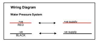
The electrical circuit should be protected with an overcurrent protection device in the positive lead.
